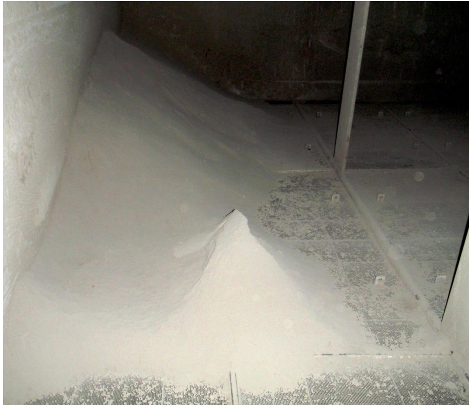
Figure 7. Acute Fouling of Large Areas of Catalyst
